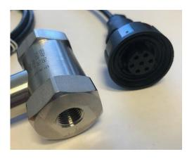
In this specific setup, the ESG-Logger-AN was fitted with a Bulgin connection.
